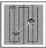
When product begins spreading, WALK over the application area at a NORMAL WALKING PACE. (6 seconds for a 25' strip, or 12 seconds for a 50' strip). CONTINUE to within 2' of the end of the application area, and begin a new row by taking 2 STEPS TO THE RIGHT OR LEFT, and walk back parallel to your first row. There should be a SLIGHT OVERLAP to the spread radius. CONTINUE in this manner until you have finished applying the product.
