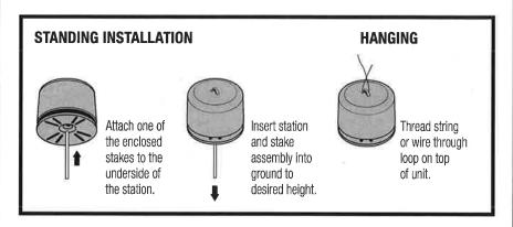
The stakes are designed to fit snugly so that wind and animals cannot easily disrupt them. Insert the other end of the stake in the ground and press down to achieve desired height.
